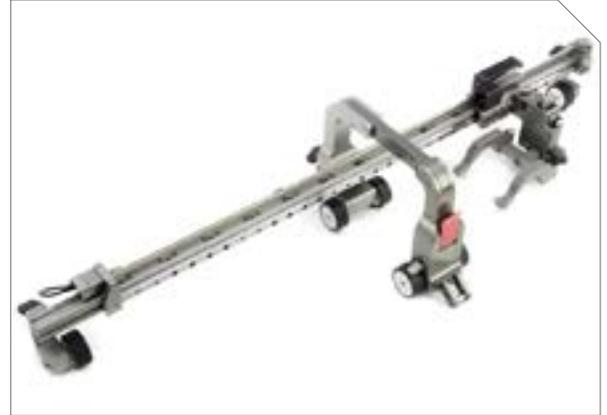
The Rotix – CEG027 is a manual chain corrosion scanner with a built in positional encoder and index encoder. It is designed to translate phased array probes and wedges around non-ferrous piping and vessels for the purpose of corrosion inspection. Urethane wheels built into the chain links provide smooth constant rolling when scanning. The Rotix chain can be adapted from 4 in. – 38 in. OD using multiple combinations of short and long links.
